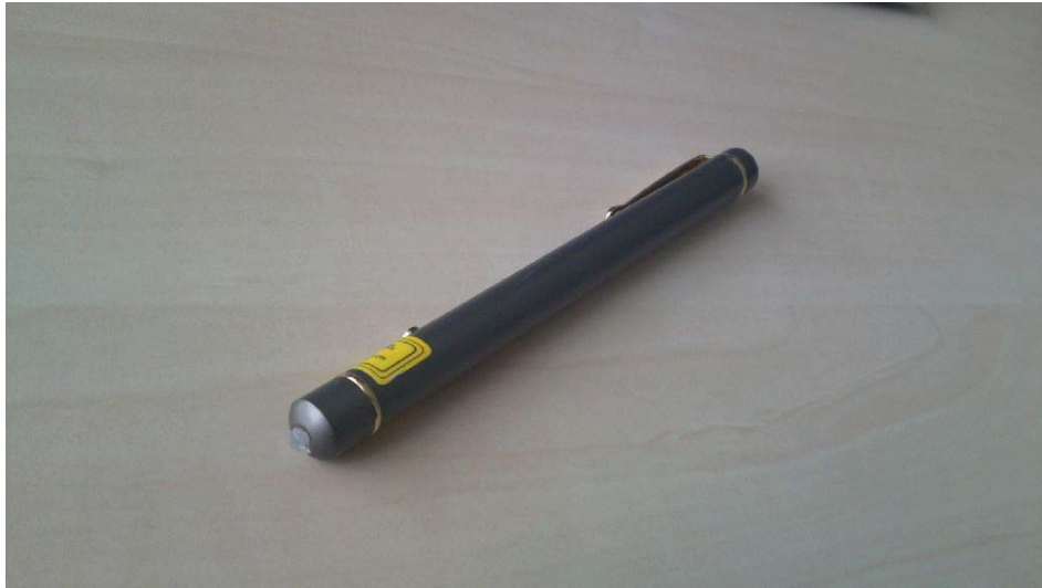
Figure 4.4: Laser pointer used for creating the point correspondences in the images. Note the little piece of plastic at the top which creates a diffuse point.
