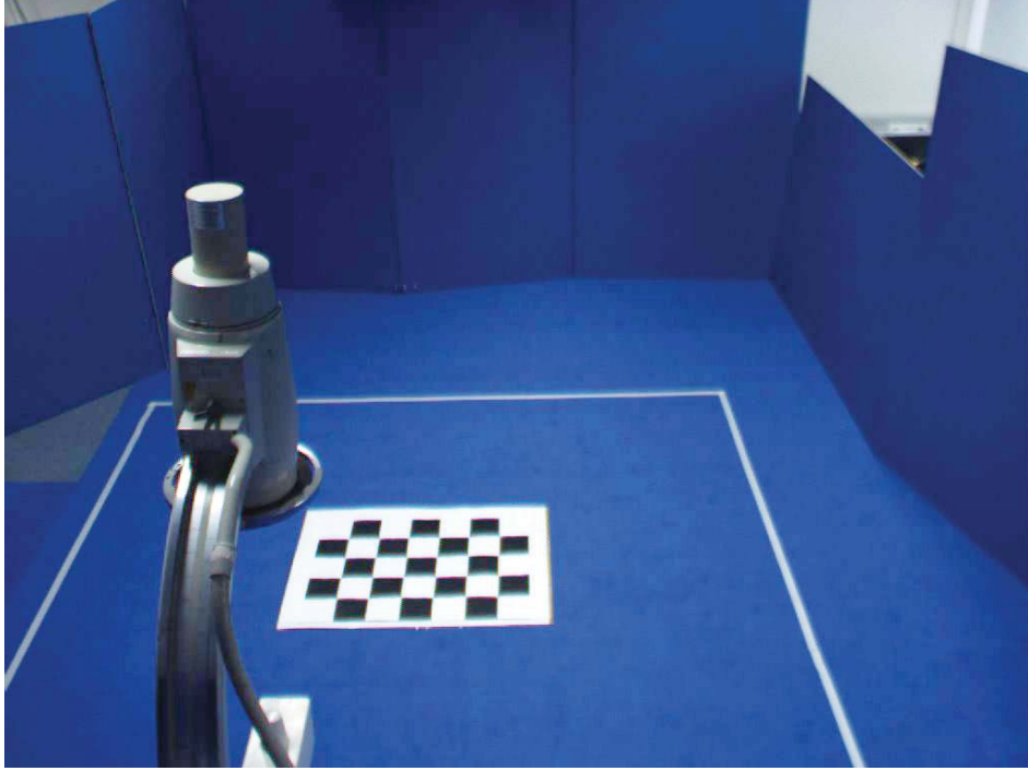
Figure 4.5: Calibration target for registering the camera coordinate system to the room coordinate system.
