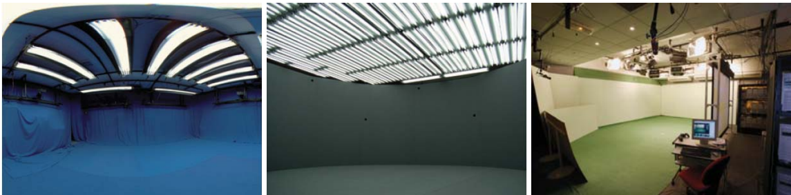
Figure 2.9: Multi-view systems at Surrey, Kyoto and INRIA respectively. Note the controlled lighting and the uniform background to improve the background subtraction results. (Images taken from [SMN + 09] and GrImage website)
