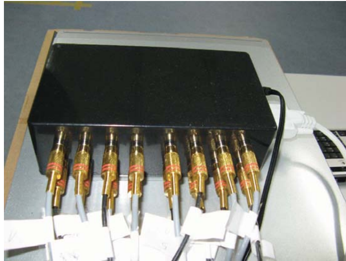
Figure 4.2: The trigger box used for synchronizing the cameras.
