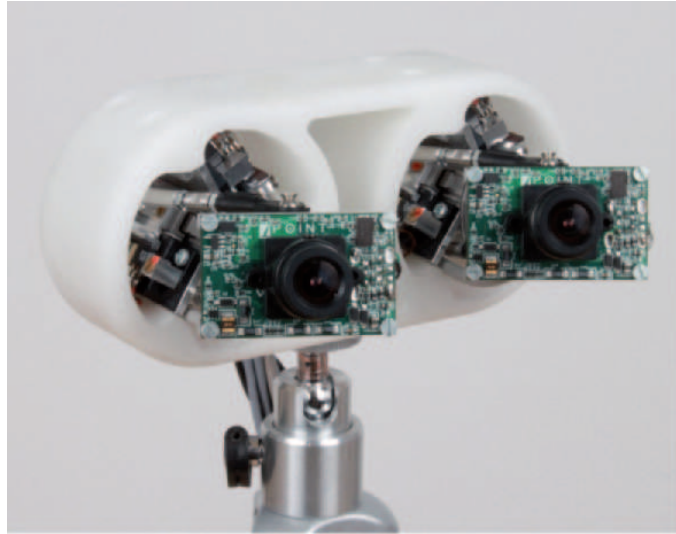
Figure 6.6.: Preliminary active vision system intended for humanoid robots; courtesy of the Institute for Cognitive Systems, TUM.
