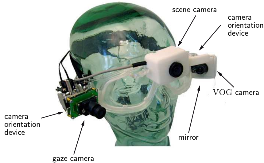
Figure 6.3.: Preliminary version of the head-mounted gaze-driven stereo camera system; courtesy of the Chair for Clinical Neurosciences, LMU Munich.
