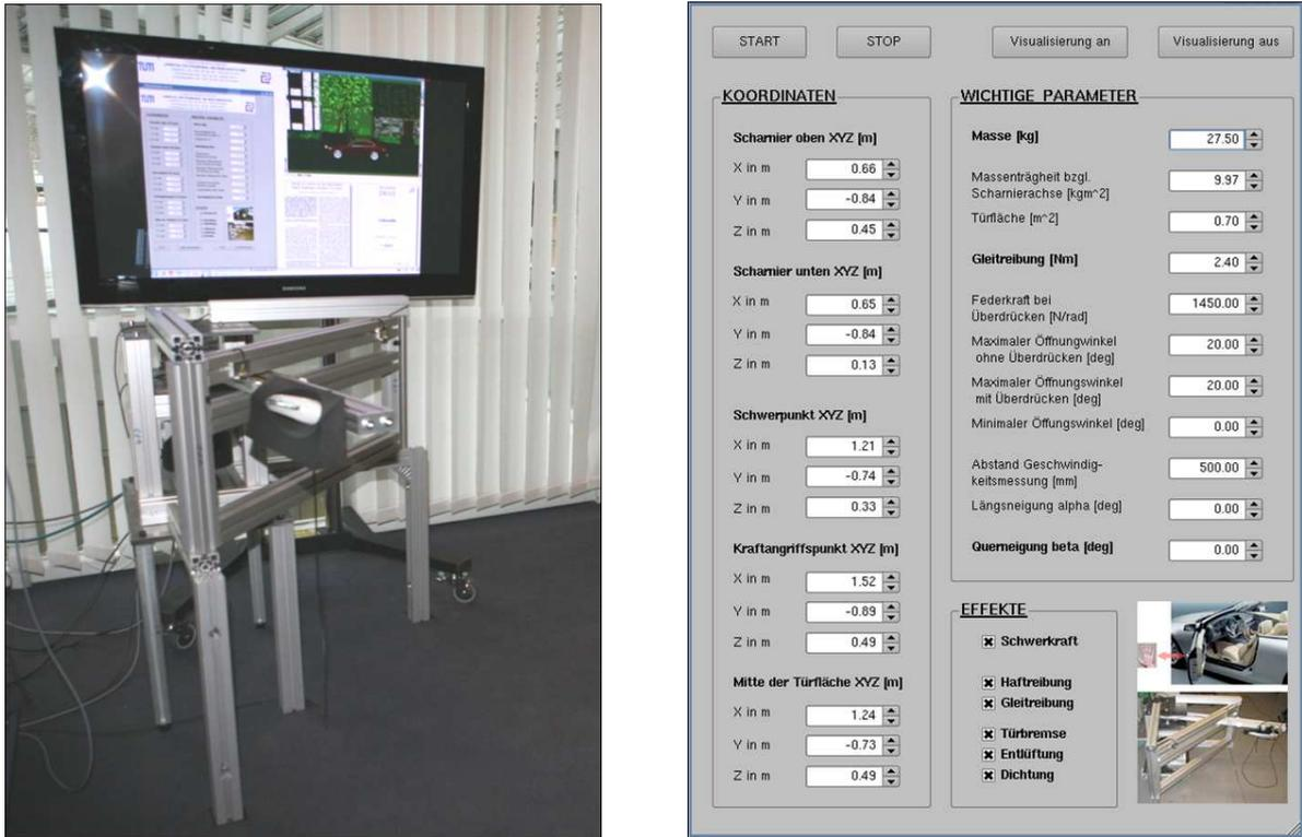
**Figure 4.19:** Setup of the high-fidelity haptic car door simulator with visual feedback (l.) and the corresponding user-friendly GUI for interactively changing simulation parameters.
