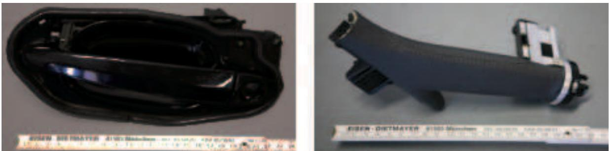
**Figure 4.2:** Inner (l.) and outer (r.) car door handles modified for use as end-effectors at the generic VRP test bed.
