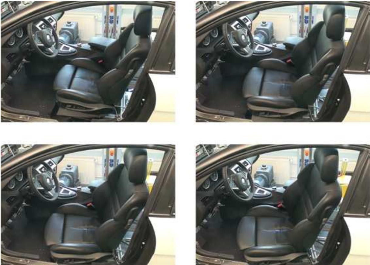
**Figure G.3:** Movement of the seat system provided by MiMed (TU München). The seat is used to decrease the level of discomfort during ingress and egress by supporting the desired motion of the driver entering/leaving the car.
