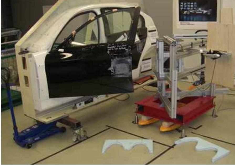
**Figure 4.20:** Experimental setup: Real door (l.) and haptic device (r.) with equally adjusted feet positioning elements for the blindfolded participants.
