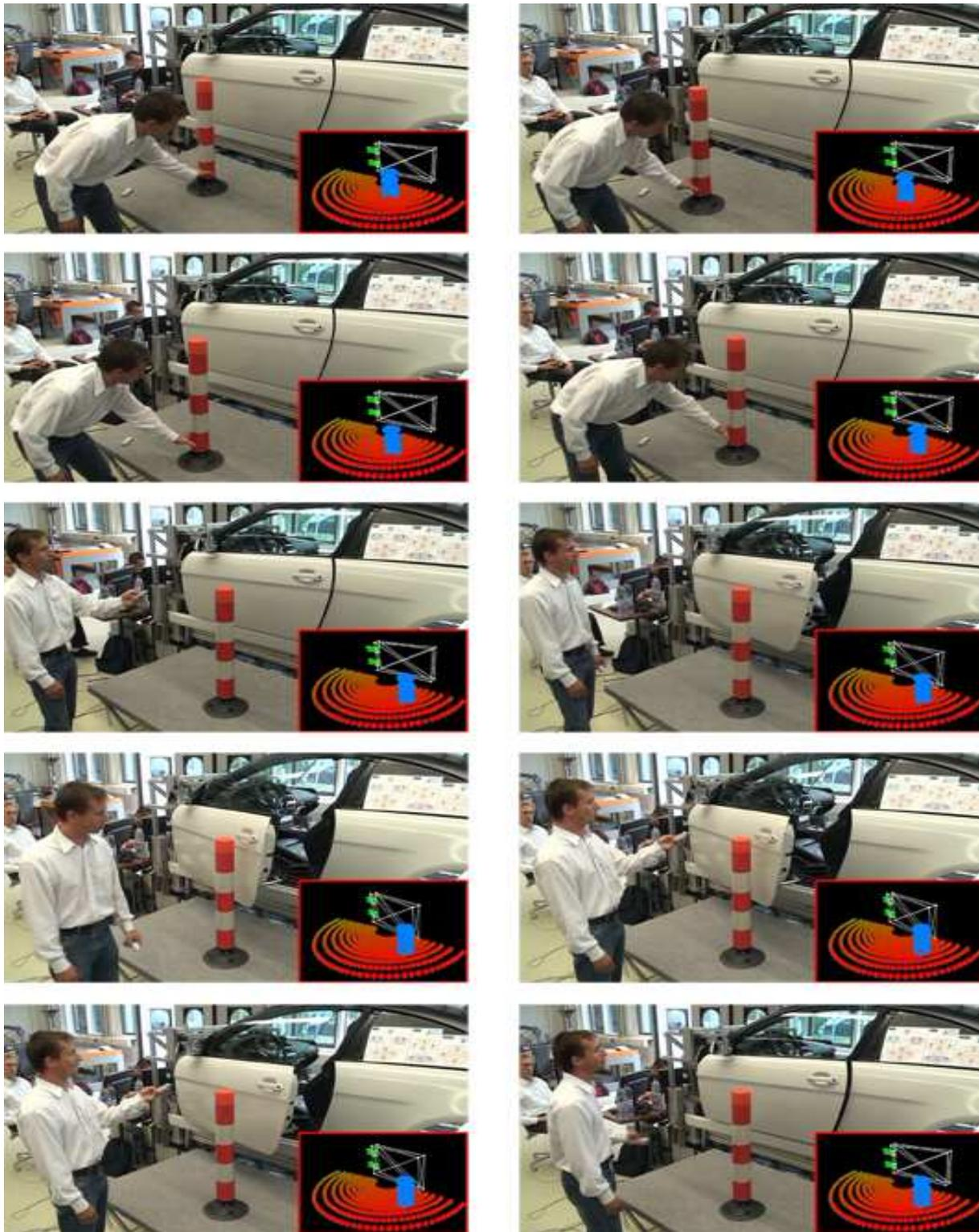
**Figure G.6:** Example of the obstacle-detection based adaptive automatic opening: Bounding boxes (blue) are generated for all 3D volume covered by potential obstacles. The effectiveness can be seen from the “tracking” of the dynamically moved obstacle. Based on this 3D data, the path planner and collision avoidance of the door controller provide a collision-free automatic opening of the door.
