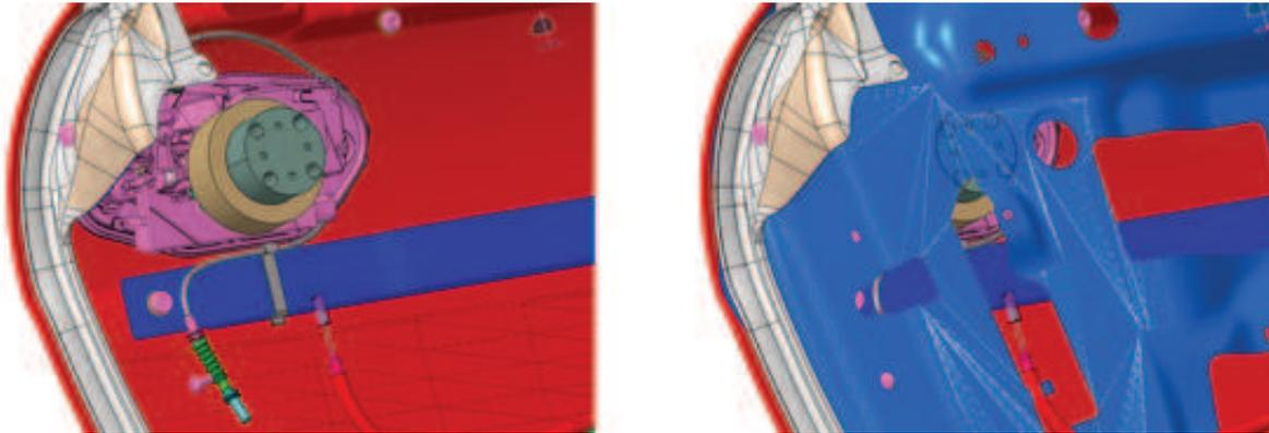
**Figure 5.3:** CAD drawings showing how the FTS was integrated into the car door body.
