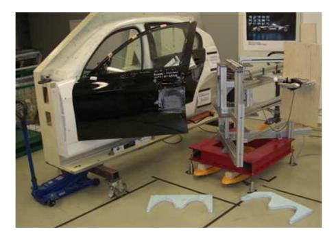
**Figure 4.20:** Experimental setup: Real door (I.) and haptic device (r.) with equally adjusted feet positioning elements for the blindfolded participants.
