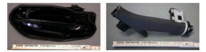
Figure 4.2: Inner (I.) and outer (r.) car door handles modified for use as end-effectors at the generic VRP test bed.
