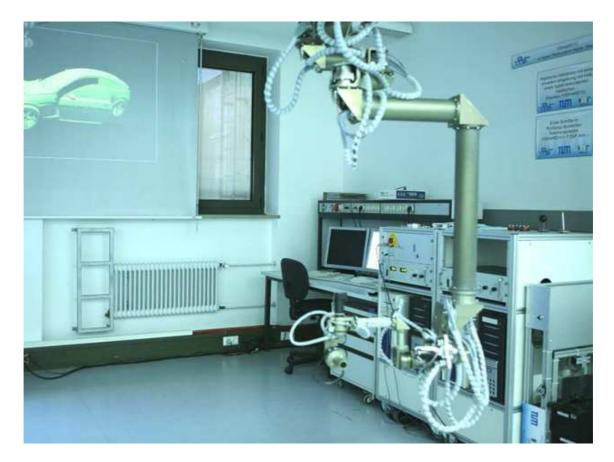
**Figure 4.1:** VRP test bed for the high-fidelity haptic rendering of actuated car doors. The virtual scene is visualized by a projector. For an improved immersion, an HMD with a head tracking system to show the correct perspective can be used.
