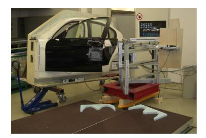
Figure 4.22: Experimental hardware setup for the investigation of the transparency of the haptic rendering of an inclined car door.
