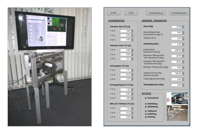
Figure 4.19: Setup of the high-fidelity haptic car door simulator with visual feedback (I.) and the corresponding user-friendly GUI for interactively changing simulation parameters.
