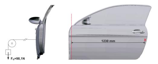
Figure 5.10: Test bed for validating acceleration measurements at a car door.
