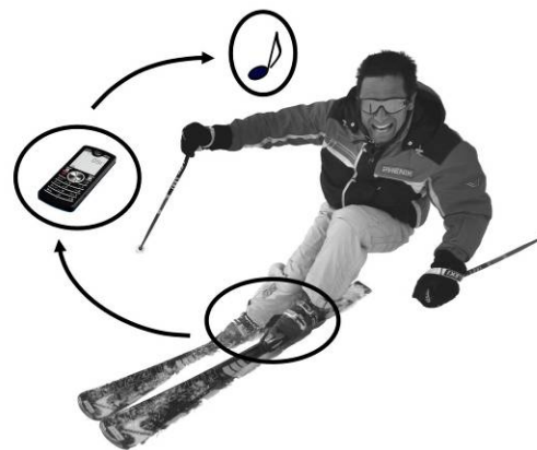
Figure 5-2: Concept of the Digital Skiing Coach: measurement of sole pressure distribution, data analysis and interpretation results in real-time audio feedback.
