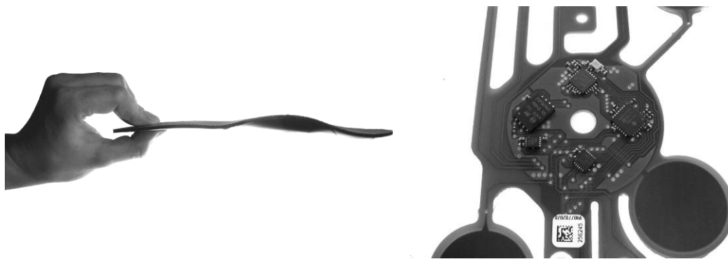
Figure 5-31: Slim, fully integrated sensor insole package (left) that incorporates a flexible circuit board, including the embedded system and the foil pressure sensors (right).
