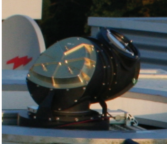
Figure 2.6: Laser Communication Terminal (LCT) with a 6.5cm aperture during the SGL experiments in Oberpfaffenhofen 2007.
