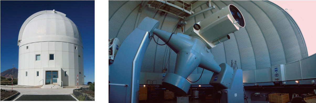
Figure 2.4: ESA OGS on the Canary island Tenerife. Left: Building of the OGS; Right: The 1m telescope with the paraxial mount.
