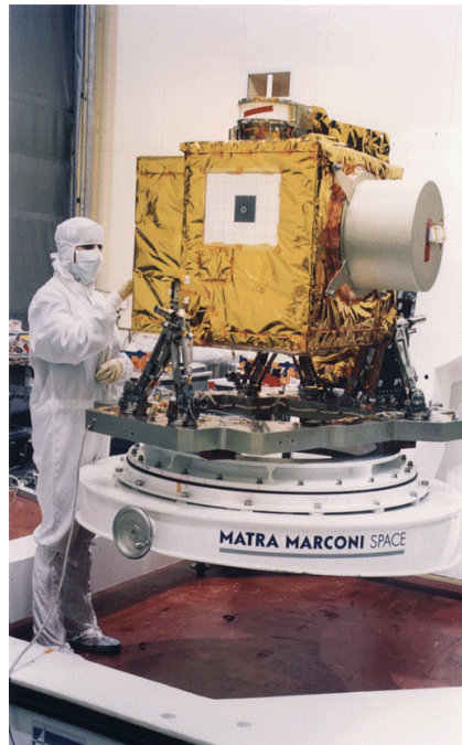
Figure 2.2: The terminal PASTEL on the geostationary satellite ARTEMIS.
