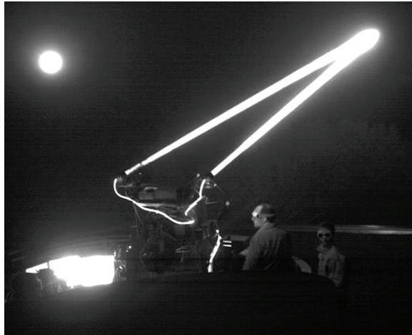
Figure 3.23: DLR OGS seen from an installed web-cam during the OICETS satellites passes 26 th June 2009 at 2:53AM local time. The two co-aligned beacon lasers on opposite sides of the telescope, which illuminate the satellite for the link acquisition and tracking, can be nicely seen. Also the glow of the fiber feed is visible.
