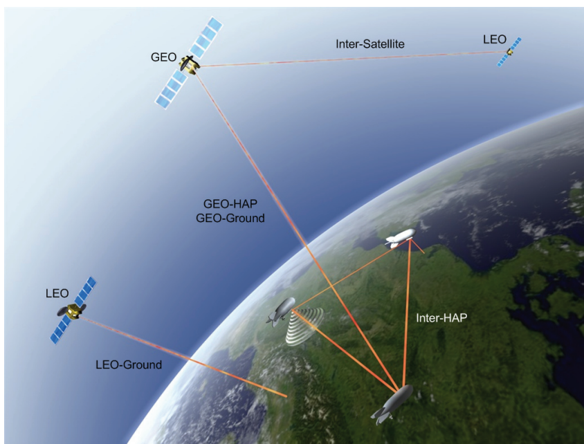
Figure 1.2: Possible link scenarios for optical communication links involving satellites and high altitude platforms (HAP).
