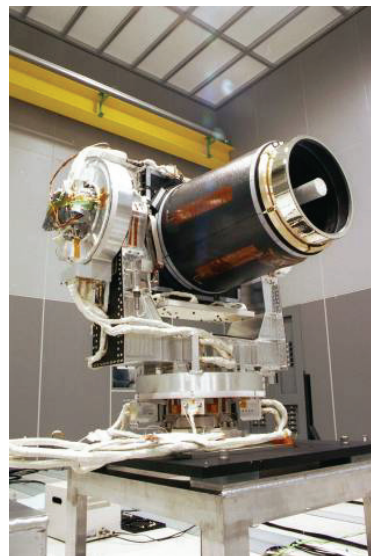
Figure 2.3: The OCT LUCE on the Japanese LEO satellite OICETS. Left: LUCE during the integration on OICETS; Right: LUCE in the laboratory.
