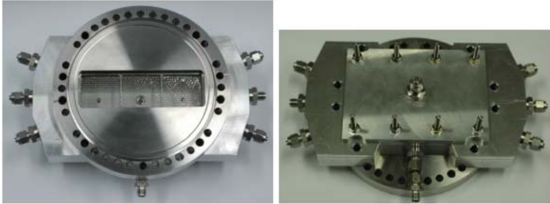
Fig. 2.14: Left: The HTM RTC viewed from the side which is attached to the separator. The supporting honeycomb structure 140 \times 40 \text{ mm}^2 can be seen. Right: HTM RTC from the other side, the many gas valves for an adjustable gas flow are visible.
