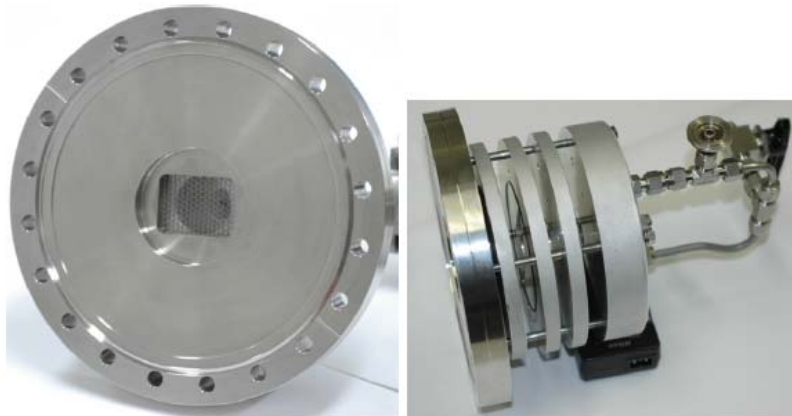
Fig. 2.15: Left: The SIM RTC with an entrance window of 30 \times 40 \text{ mm}^2 . Right: Side view of the SIM RTC. Spacers can modularly be introduced to the setup to change the depth of the RTC.
