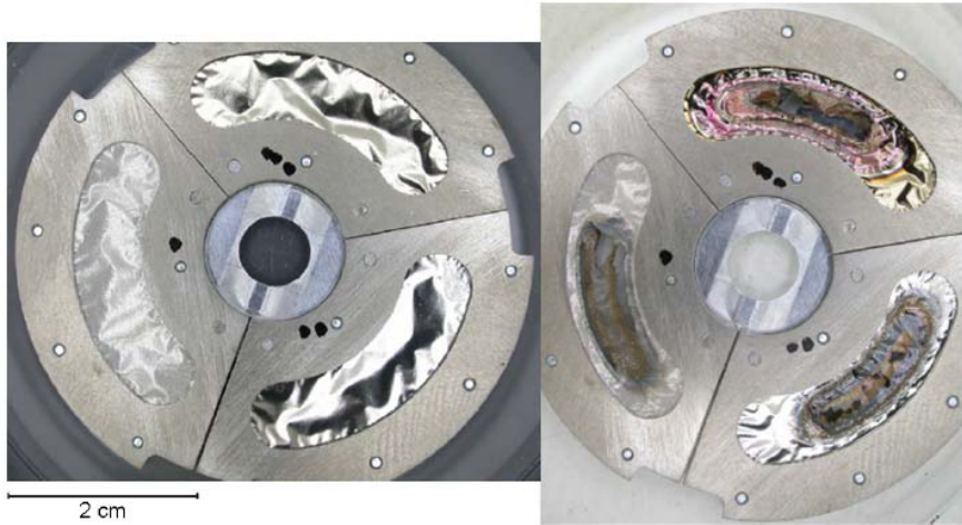
Fig. 2.8: Pictures of the front side of ARTESIA mounted with ^{238}\text{U} target material. Backing/target material/fronting: left: C/U/C, top: Ti/U/-, bottom: Ti/U/C. The left picture was taken before, the right one after irradiation.
