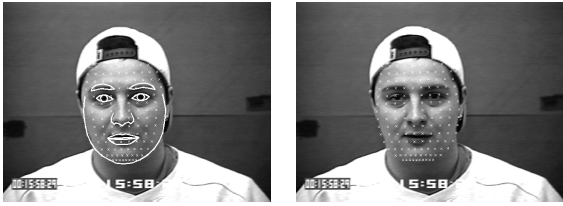
Figure 5: Model-based image interpretation for facial expression recognition: Fitting a deformable face model to images and inferring different facial expressions by taking structural and temporal image features into account.
