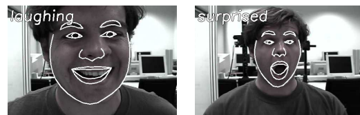
Figure 1: Model-based techniques greatly support the task of facial expression interpretation. The parameters of a deformable model give evidence about the currently visible state of the face.
