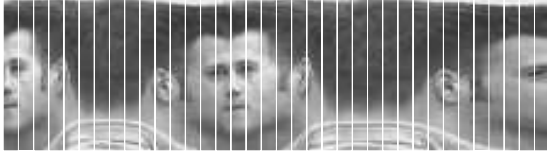
Fig. 6. Image for the initialization of the model during training, at least a full rotation is trained on the loop of column-models. Those images are generated by concatenating image columns over time
