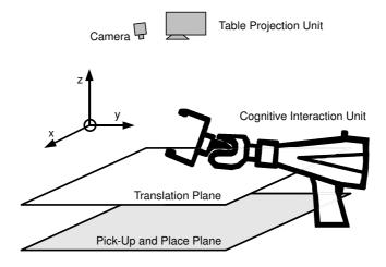
Fig. 1. Overview of the working x-y-planes
