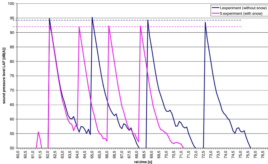
**Figure 3:** Comparison of the A- and Fast-weighted sound pressure level
