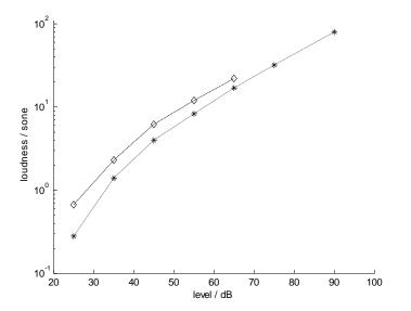
Figure 1: Loudness of pink noise as a function of its overall level. Rhombs connected by dashed lines represent loudness data given in ANSI S3.4-2007; stars connected by dotted lines indicate loudness data calculated according to DIN 45631 (1991).
