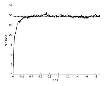
**Figure 3:** Loudness-time function for the sound of a planing machine (solid) calculated according to DIN 45631/A1 (2008) in comparison to the loudness value (dotted) calculated according to DIN 45631 (1991).
