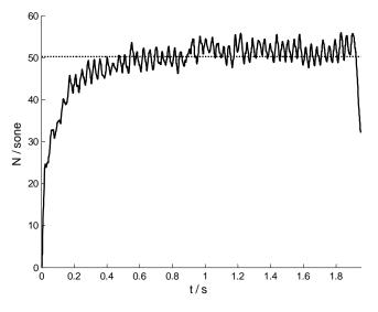
**Figure 4:** Loudness-time function for the sound of a jackhammer (solid) calculated according to DIN 45631/A1 (2008) in comparison to the loudness value (dotted) calculated according to DIN 45631 (1991).
