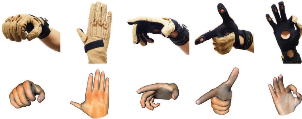
Figure 5.4: Gesture mapping from real human hand to virtual hand model.
