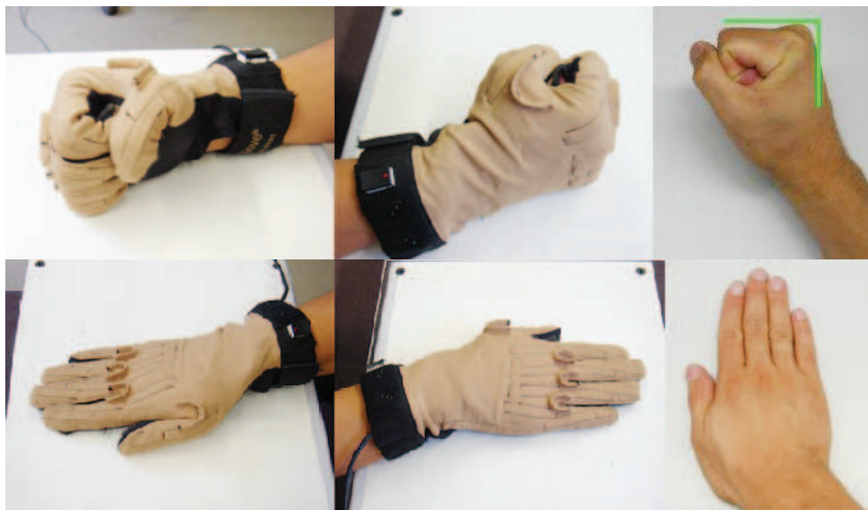
Figure 6.1: Quick calibration procedure for the CyberGlove.
