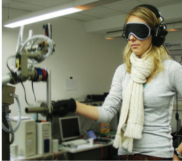
Figure 7.1: HRI experiment: a blind-folded subject wearing sound-prove headphone shakes hand with the robot.
