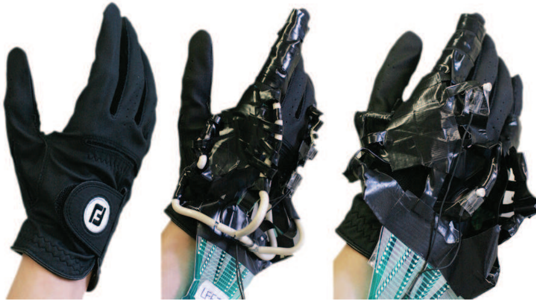
Figure 4.6: Base glove without sensor, TSG2 design 1 with manufacturer suggested sensor layout, TSG2 design 2 with customized sensor layout.
