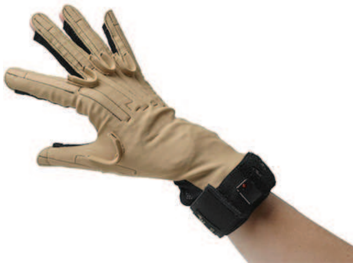
Figure 4.1: CyberGlove with 22 sensors to measure human hand gestures.
