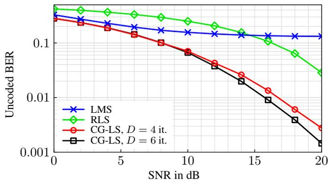
Fig. 4. BER comparison with LS based CG method when starting algorithms with zero vector
