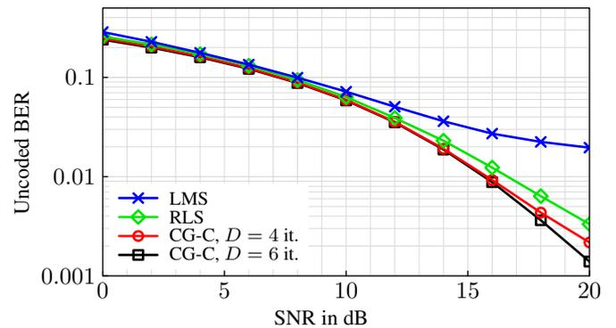
Fig. 3. BER comparison with correlation based CG method when starting algorithms with filter vector of the previous block
