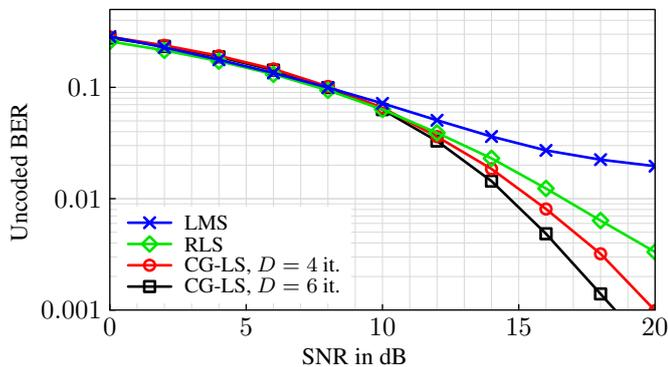
Fig. 5. BER comparison with LS based CG method when starting algorithms with filter vector of the previous block
