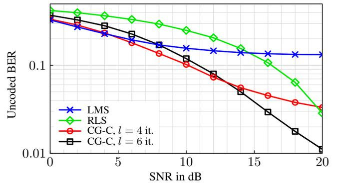
Fig. 2. BER comparison with correlation based CG method when starting algorithms with zero vector
