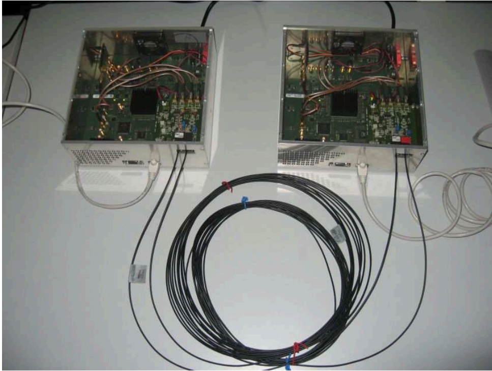
Figure 7.1: Test bed of two connected Gigabit Ethernet media converters with a fiber length of 10 m.
