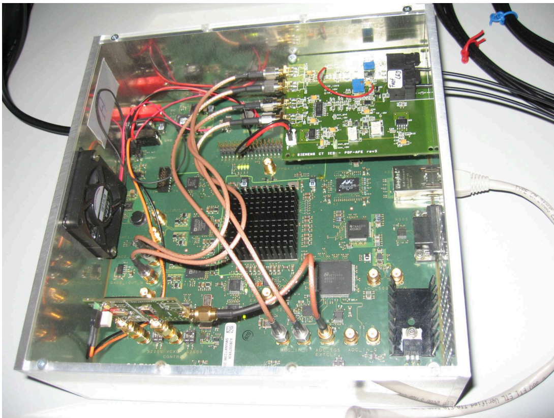
Figure 6.21: Gigabit Ethernet media converter.
