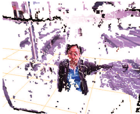
Figure 2.3: Stereo vision data comes in ‘depth slices’ that are spaced unevenly across the covered range. While depth accuracy may be on the order of millimeters for close-by objects, it deteriorates to up to 10 centimeters for objects that are several meters away. The point cloud shown in this figure was recorded with a Bumblebee 2 on the system described in [166].
