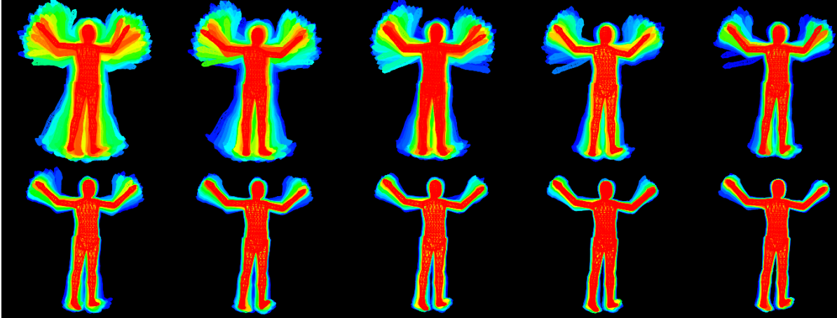
FIGURE 4.6 Visualization of the particle set during the iterations of the annealed particle filter (for 10 layers). Particles are rendered with their corresponding pose estimate. Higher color temperature corresponds to higher weights. With each iteration, diffusion is reduced and particles eventually cluster around the global maximum.
