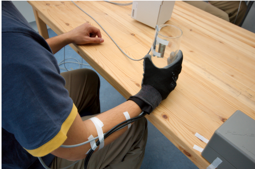
FIGURE 2.5 Magnetic system for marker-based motion capture. In this example, the system is used to record grasping motions. The glove is equipped with several markers to detect the articulated pose of the hand. Image courtesy of Alexis Maldonado, TUM.
