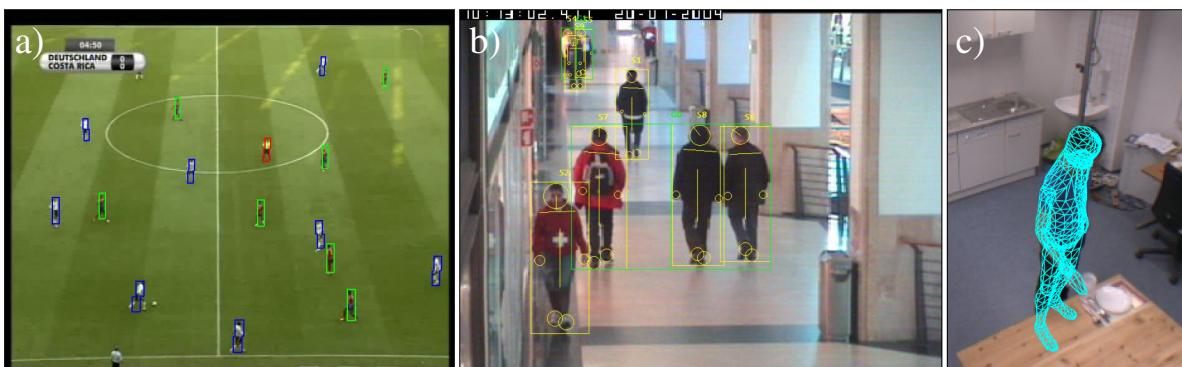
FIGURE 1.1 Different application scenarios for human observation: a) tracking of soccer players from TV broadcasts (image taken from our earlier work on sports analysis [19, 22, 60]) b) pedestrian detection for surveillance or safety applications (image with marked up ground-truth taken from the PETS 2004 CAVIAR data set [118]) c) fullbody tracking of human manipulation activities in living environments (as presented in this thesis). Notice the increasing level of body details that are being estimated from Figure a to c.
