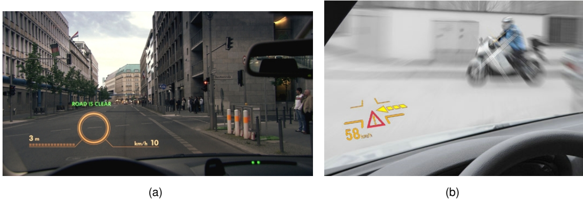
Figure 5.51: Possible futuristic Intersection Assistance systems using C2X technologies (a) a visualization suggested within [EUCAR] project, (b) visualization from BMW ConnectedDrive project [BMWPressclub]. For these functionalities all vehicles have to be equipped with C2X technologies
