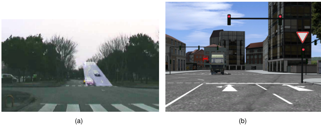
Figure 5.52: Presentation of occluded objects at intersections with C2I technologies (a) visualization of one Japan intersection equipped with cameras [Taya05], (b) possible visualization from [Plavsic09b]. For these functionalities not all vehicles have to be equipped but the driven vehicle and intersection infrastructure
