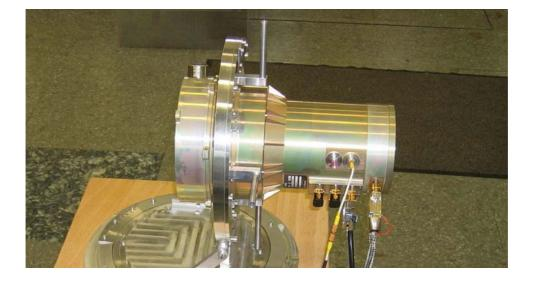
**Figure 2.8:** *Top panel*: Schematic cross–section of a GBM NaI detector showing the main components. A picture of a detector flight unit mounted on the calibration stand was taken in the laboratory during detector level calibration measurements and is shown in the *bottom panel*
