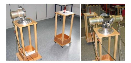
**Figure 3.1:** Detector holders with NaI (*left panel*) and BGO detectors (*right panel*) are positioned in front of the radioactive source (on top of the red holder) on their wooden stands during the calibration at the MPE laboratory
