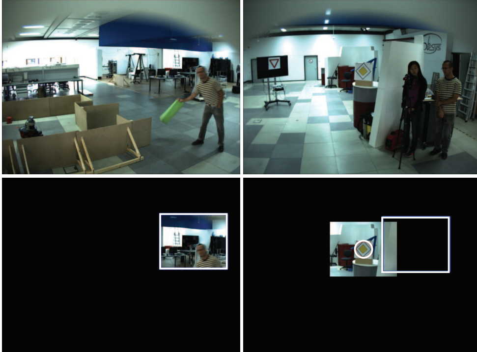
Fig. 4.14: Left column: bottom-up state; Right column: top-down state; Upper images: original input images; Lower images: the resultant robot attention windows. Rectangles: the salient/surprising image regions (the same as the masked region in bottom-up state); Masked regions: the current robot FOA; Circle: the detected target object.
