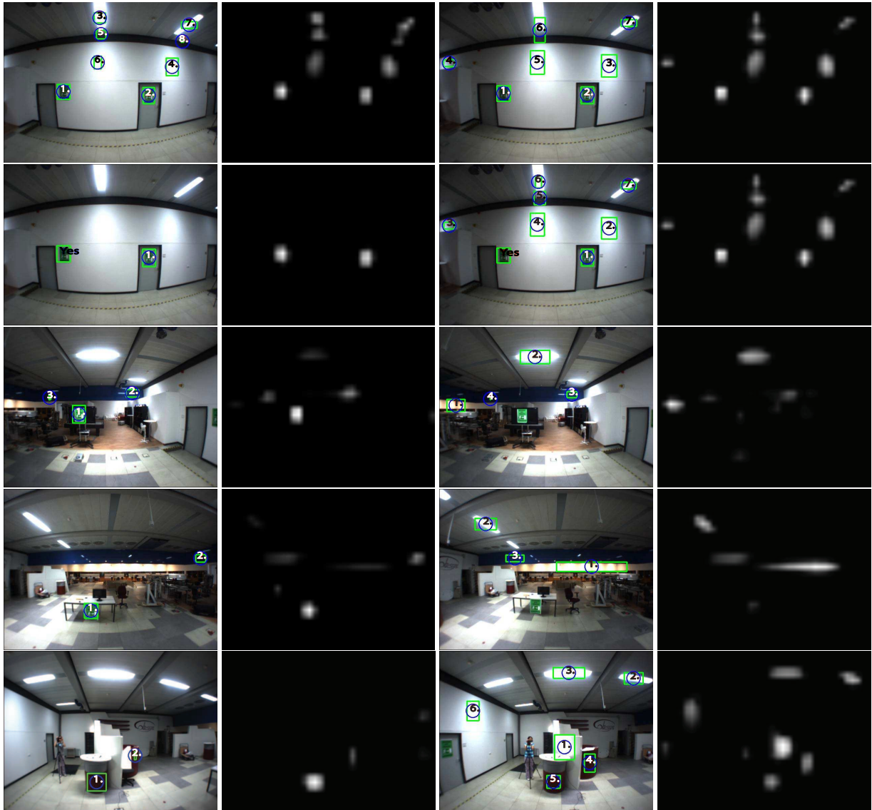
Fig. 4.4: Column 1: object maps predicted using B1T1K1; Column 2: saliency maps computed using B1T1K1; Column 3: object maps predicted using B1T0K0; Column 4: saliency maps computed using B1T0K0. Numbers on the object maps indicate the fixation sequence along with a descending saliency value of the selected image region candidates. “Yes” on the object maps indicate that an image region candidate contains a target object.
