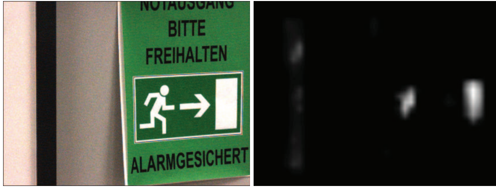
Fig. 4.11: Saliency map computed directly from a sample image. Left: sample image. Right: the respective saliency map.
