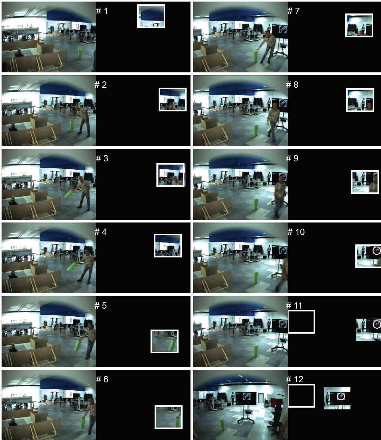
Fig. 3.10: Image sequence for object detection task. Left sub-columns: the original input images. Right sub-columns: the respective masked result images with the frame number. Masked regions: the robot FOA; Rectangles: image regions containing the maximum LS; Circles: the detected objects.
