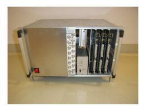
**Figure 6.13:** Electronic system for the MADPET-I lab course, including all power supplies (low-voltage, high-voltage), rotating table control and three SADC modules with USB readout (*right*). [Sch09]
