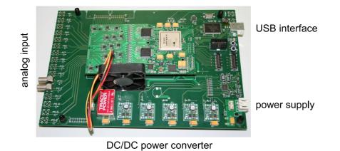
Figure 5.17: USB interface for the MSADC module.
