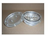
**Figure 6.16:** Sample source for the lab course with the TUM logo as active region. The source is milled from plexiglas and can be filled with <sup>18</sup>F-FDG. [Sch09]
