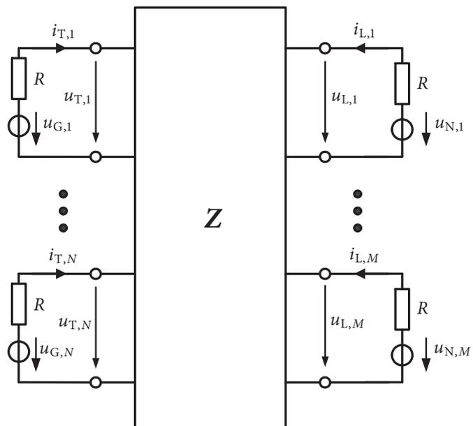
Figure 2: Circuit theoretic multi-port model of a linear multi-input multi-output communication system, with signal voltage generators, load terminations, and noise voltage sources.
