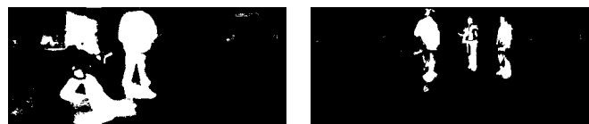
Less noise in background modeling based on [17], but still detected shadows pixels.
