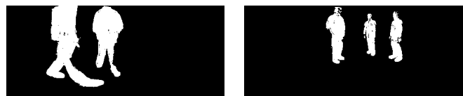
Our approach with proposed shadow and foreground detection. Noise as well as shadows can be better suppressed.
