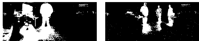
Foreground detection using Mixture of Gaussian and low thresholding results misclassification (shadows, noise).
