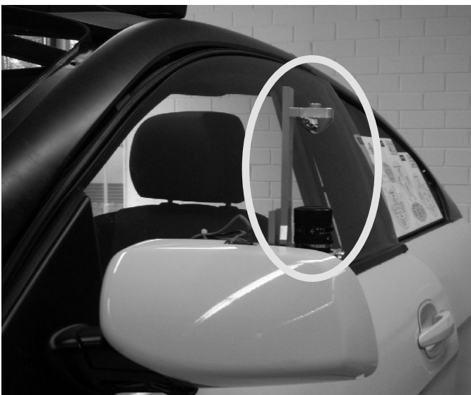
Fig. 3. Our camera system integrated with the side-view mirror of a car.
