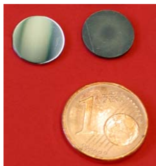
Figure D.1.2: Polished and sandblasted surgical stainless steel blanks.
