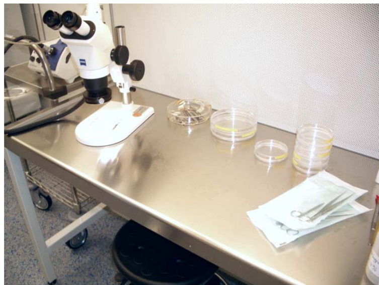
Fig. 2.27: Dissection hood 2. Here dissecting microscope and other dissecting supplies can be seen. All supplies and surfaces should be thoroughly sterilized prior to preparation and dissection.
