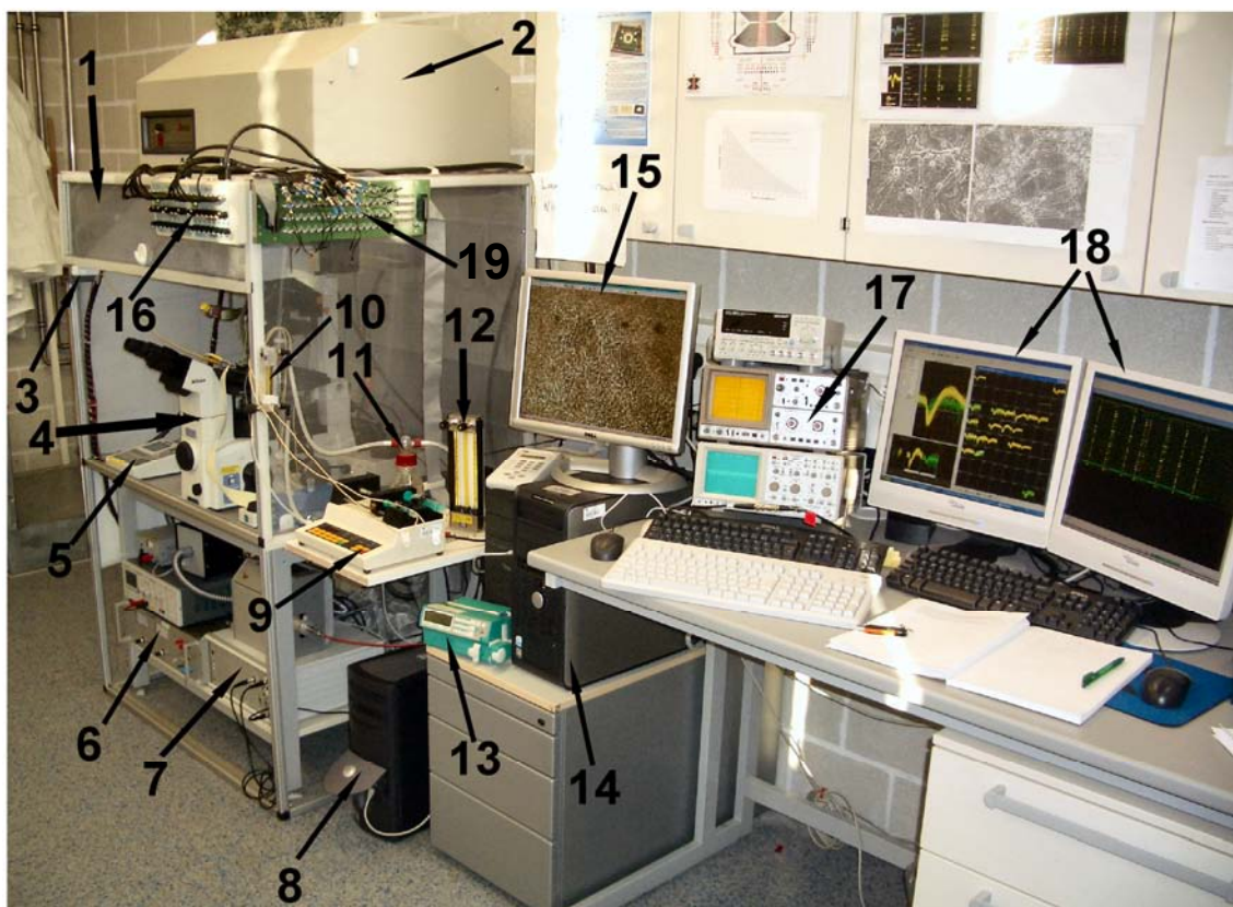
Fig. 2.45: Workstation for neuro-electrophysiological experiments showing all the necessary life-support and data acquisition equipment: 1) Faraday cage, 2) HEPA air filter unit, 3) Temperature controller for cell culture chamber, 4) Inverted phase contrast/fluorescence microscope, 5) Manual control pad for microscope, 6) Power supplies for heating and stimulation devices, 7) Control unit and monochromator for fluorescence microscopy, 8) Microscope control PC, 9) Precision syringe pump for osmolarity maintenance, 10) Low-volume gas flow meter, 11) Gas humidification bottle, 12) CO 2 /air mixing controller, 13) Infusion pump, 14) Plexon data acquisition PC, 15) Live cell culture display, 16) 16-channel pre-amplifier/filter system for audio output of electrical activity, 17) Analog/digital storage oscilloscopes for variable-resolution (temporal) activity display, 18) Activity display, 19) 64-channel Plexon BNC board for connection of analog signals to audio amplifiers.
