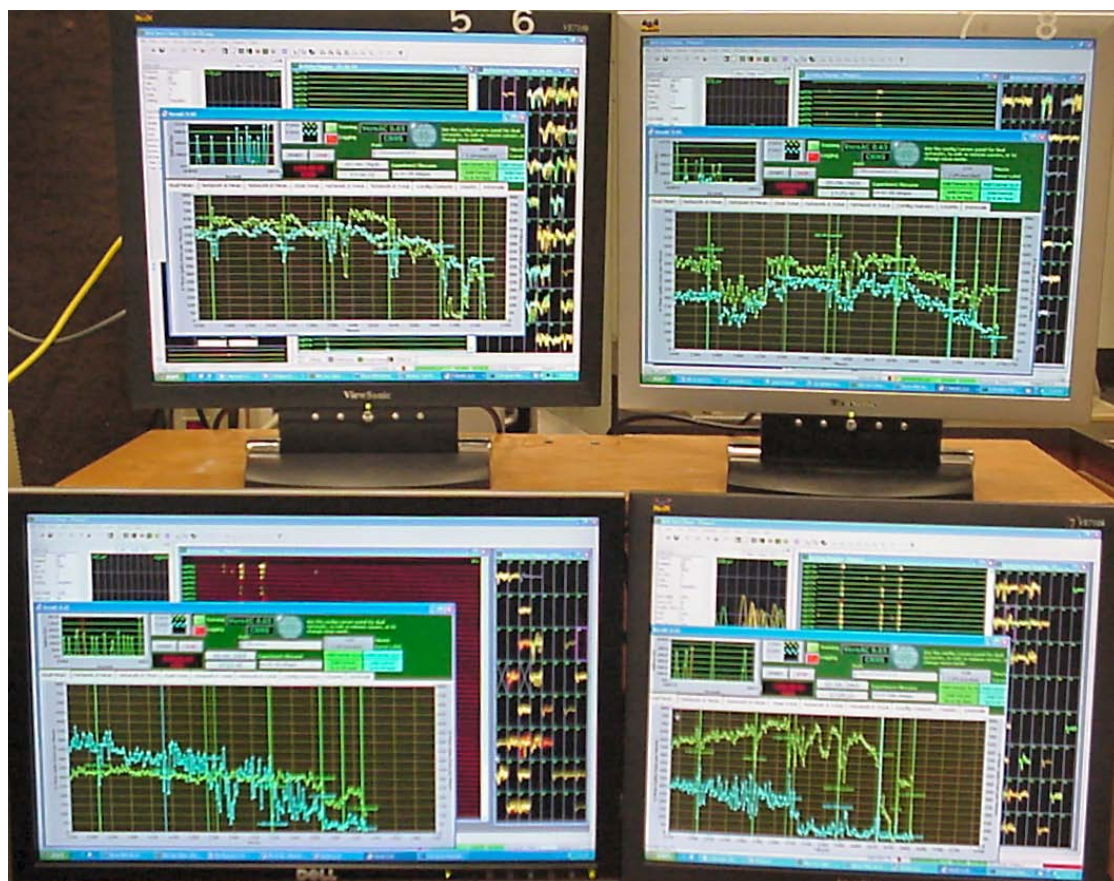
Fig. 4.92: Simultaneous recording of 8 separate networks using 4 PCs: Plexon Sortclient software, and CNNS custom made program “VernAC”, based on LabView.
