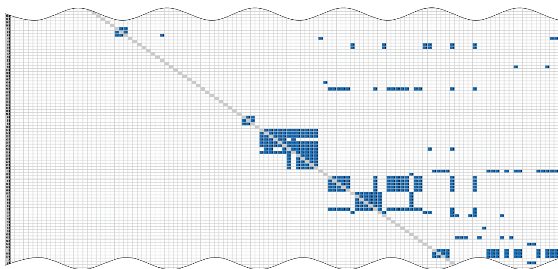
Figure 7-18: Section of the activity-activity DSM (via documents) exhibiting 74 feedbacks after triangularization
