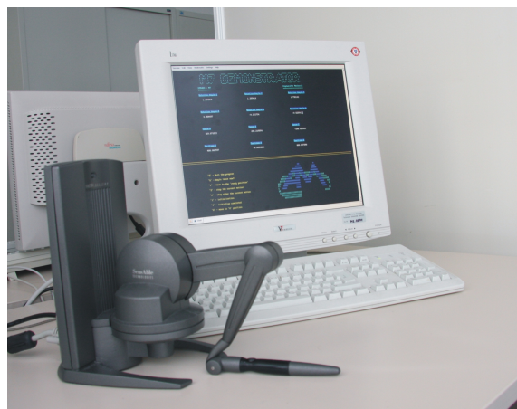
Figure 6.5.: Phantom Desktop. The computer screen shows the interface of the robot motion control system.
