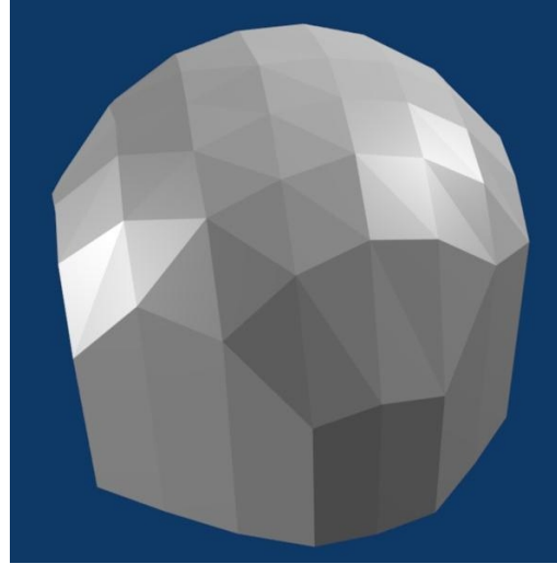
Figure 6.25.: The Geometric model of the Sphere. After the surface reconstruction using these points, the closed surface is created, and the final geometric model with mesh has the same aspect as the closed surface.
