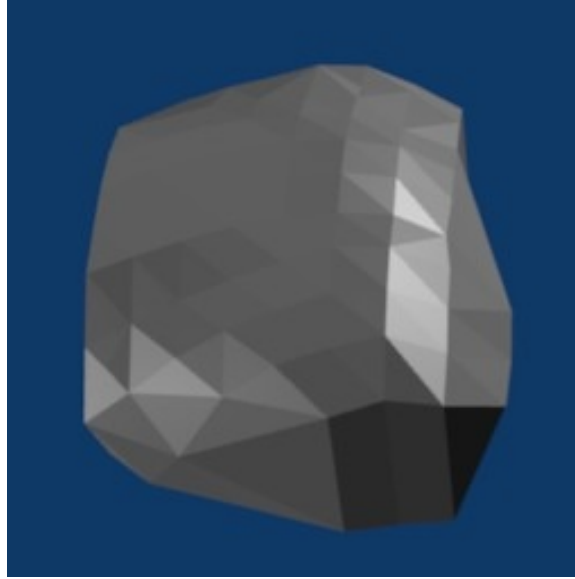
Figure 6.31.: The geometric model of the heart. Its aspect is the same as that of the closed surface after the triangulation. The contour of the model in this experiment is relative rough, because the computational expense of the model is limited by the actual experimental computer. In robotic surgery using the identical modeling method, models are generally created based on the measurements from a CT. With high-end hardware, the computing power can be sufficient for the evaluation of more complex models.
