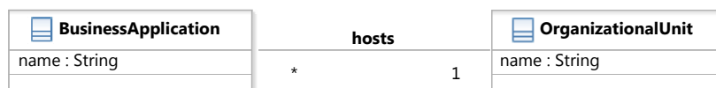
Figure A.8.: Information model fragment for I-Pattern BUSINESS APPLICATION AND ORGANIZATIONAL UNIT RELATIONSHIP
