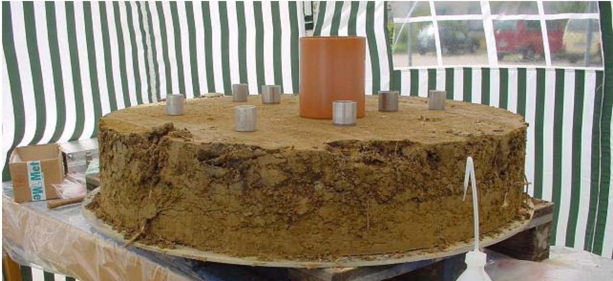
Figure 8 Single soil slice (20 cm thickness) before sampling after cutting of the soil monolith, with steel rings for bulk density determination on top.
