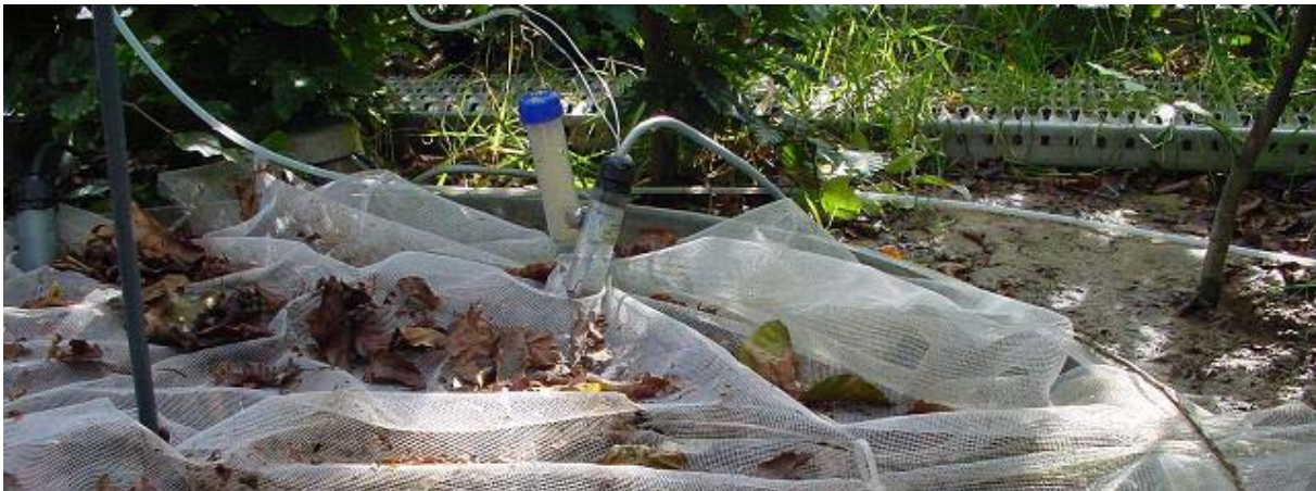
Figure 7 View on the top of a single lysimeter after cutting of beech ( Fagus sylvatica L.) trees while the final harvest in September 2006 with visible mesh and instrumentation for matrix potential measurements.
