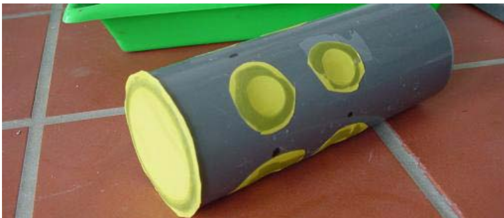
Figure 4 Sample tube capped with polyester fibre used for incubation experiments (see p. 29).
