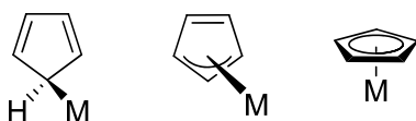
Figure 6 From left to right: \eta^1 , \eta^3 and \eta^5 coordination modes of the cyclopentadienyl ligand to a given metal.
