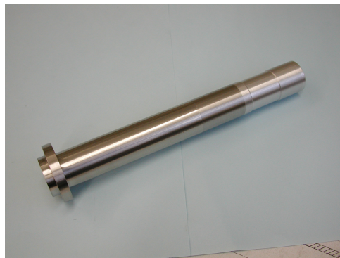
Figure F.14: Centre tube extension for the one Kelvin cryostat. The aluminium-stainless steel friction-weld has an inner diameter of 23 mm and an outer diameter of 25 mm (only 24 mm at the lower end, where the neutrons penetrate the tube).
