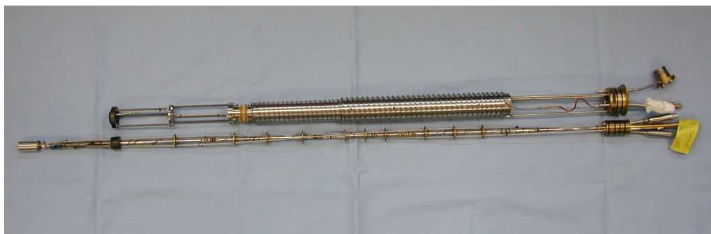
Figure F.15: 1 Kelvin ^4\text{He} evaporation cryostat inserts (compare Fig. 5.29). Above: evaporation insert with a total length of approximately 97 cm. Below: microwave insert with a total length of approximately 116 cm.
