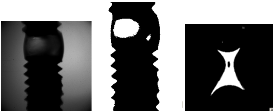
Figure 3.9.: Image processing for Fluid Filament diameter determination: Left, original image. Middle: After Black-white conversion. Right: After background subtraction (later in the movie).
