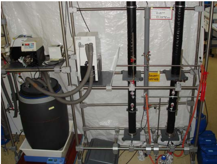
Figure 2-3: Schematic drawing (dimensions in cm) and photo of the experimental setup for comparison of slow sand filter (SSF) and intermittent sand filter (ISF) at laboratory scale
