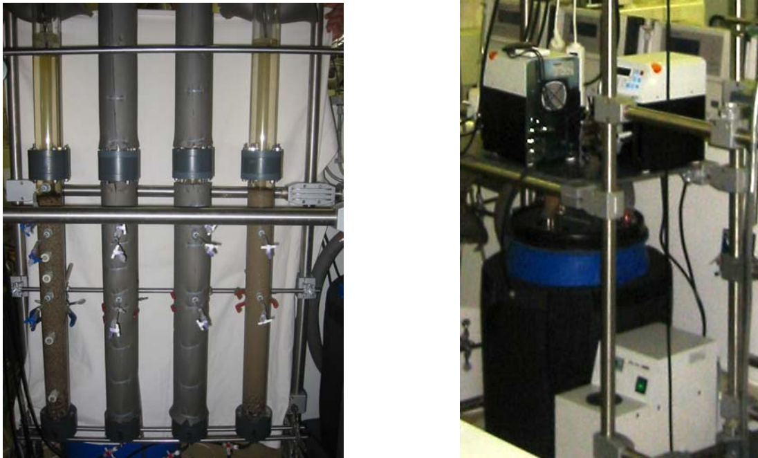
Figure 2-1: Laboratory installation of the 4 slow sand filter columns C1–C4 as well as the storage barrel, pumps and cooling unit
