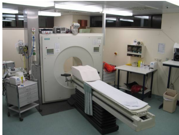
Figure C.2: Siemens ECAT EXACT HR+ PET scanner. Since the introduction of PET/CT scanners in the clinic and their clear advantage for oncological examinations, the HR+ scanner is used mainly for neurological and cardiac examinations.
