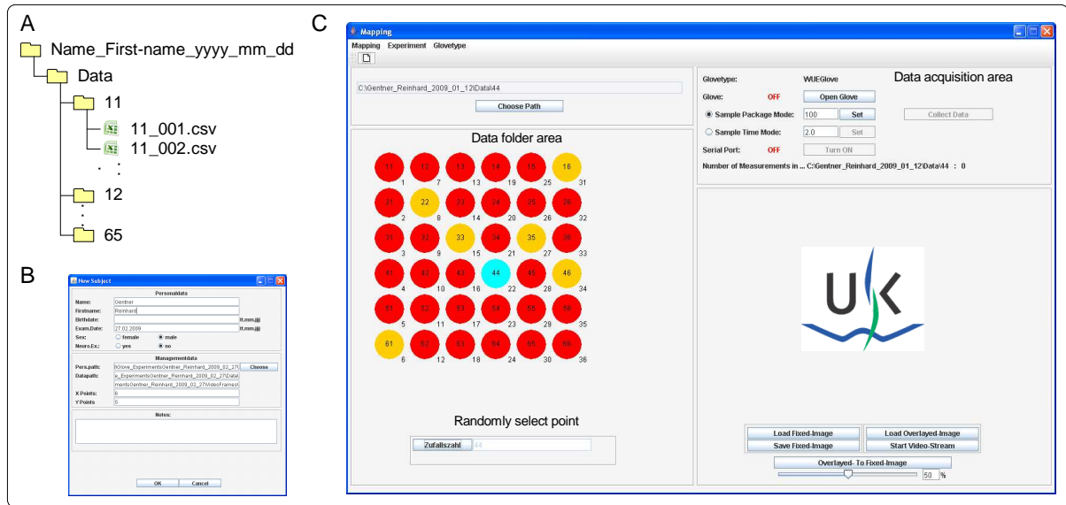
Figure 30: (A) Data structure for storage of TMS-evoked movements. For each grid point, a corresponding data folder exists. (B) Graphical user interface mask to set up the data folders and store information on the subject. (C) Main user interface for stimulation. A new stimulation point can be selected manually by clicking on the circles or randomly by the computer. Orange circles denote already stimulated points and the blue circle is the currently selected point. Sensor glove recordings can be triggered by signals at the RS232 port.
