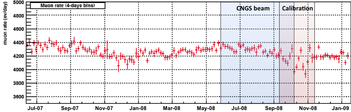
Figure 6.1: Temporal variation of the muon rate as measured by the MTB flag over the duration of 1.5 years in BOREXINO [115]. For the first year, the normal seasonal variation of \pm 2\% is visible [114]. Later on, the muon events caused by the CNGS beam and the calibration phase of BOREXINO disturb the signal.
