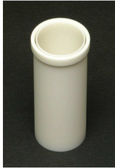
Figure 3.5: Crucible consisting of two \text{Al}_2\text{O}_3 cylinders, resulting in a sample geometry of a hollow cylinder with an outer diameter of 22 mm and a wall thickness of 1.2 mm.
