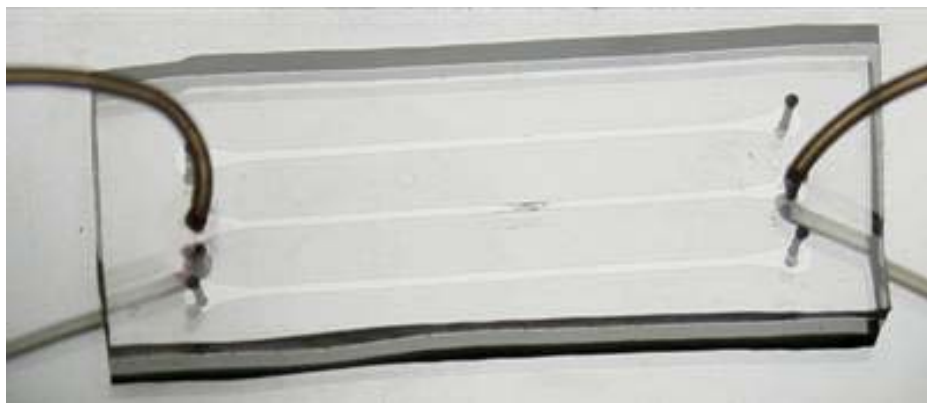
Figure 2.3. Image of microfluidic device with three microchannels in parallel. At the middle microchannel there are the inlet and outlet connected with the tubing in both extremities.
