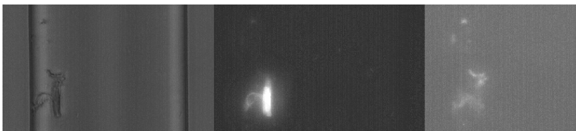
Figure 35 Bright-field image of biofilm in 100 \mu\text{m} wide microchannel after five days (left, scale bar 10 \mu\text{m} ); fluorescent micrographs with DAPI and FITC-ConA staining as observed with DAPI-filter (middle) and FITC-filter (right)
