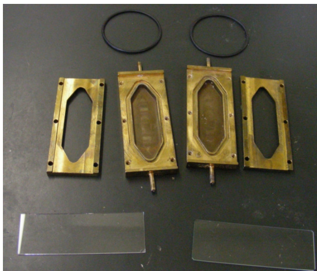
Figure 8 Two unassembled copper flow cells with rubber O-rings which can be inserted into the bottom part (middle); two glass slides (7 x 3 x 0.1 cm, shown at the bottom) can be inserted into the flow cells for biofilm growth
