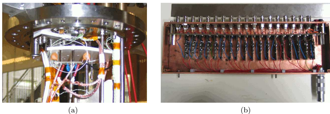
Figure 5.4: Front-end electronics in GII: (a) high voltage filters and coupling capacitors and (b) pre-amplifier box for a segmented detector.
