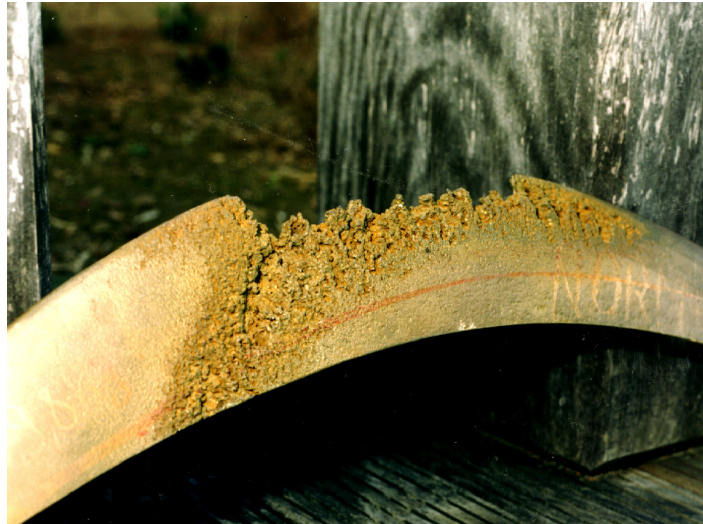
Figure 1.12: Detail of an eroded ship propeller [58].
