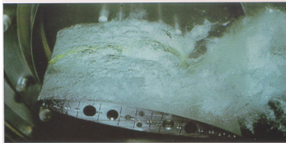
NACA 16012 Re_c = 10^6 , \alpha = 11^\circ \sigma_{ref} = 0.81 , c=0.1 m
