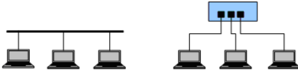
Figure 2.2: Bus and star topologies realized by the Ethernet technology
