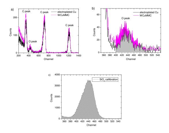
Figure 6.20: a) NRA protons spectrum of W<sub>f</sub>/Cu MMC with interface concept C and of electroplated Cu bombarded with 2.5 MeV 3He<sup>+</sup>; b) Curve integral of the O peak of W<sub>f</sub>/Cu MMC and of electroplated plus heat treated Cu to extract the O content of the samples; c) Curve integral of the O peak of the reference SiO<sub>2</sub>sample
