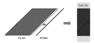
Figure 5.2:  $\pm 45^{\circ}$  fiber alignment around the CuCr1Zr cooling tube
