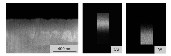
**Figure 6.4:** Resolved Cu and W signal of continuously graded W/Cu coating (interface concept concept E without annealing at 800°C) measured by EDX
