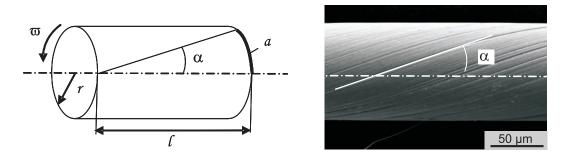
**Figure 5.1**: Defined twisting angle on the W fiber, adjusted by the number of rotations of the turning lathe
