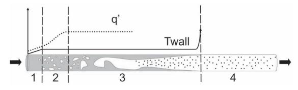
Figure 5.4: Heat transfer regimes in a uniform heated tube:
