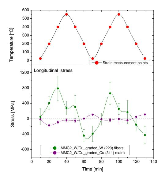
Figure 6.23: Residual stresses of fibers and matrix of MMC 2 measured by neutron diffraction
