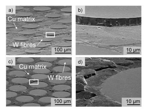
Figure 6.21: SEM images of the two investigated MMC discs after thermal cycling:
