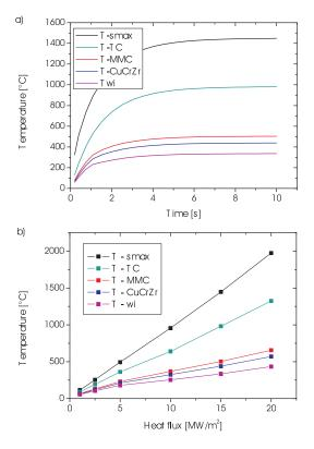
Figure 8.2: a) Temperature evolution as function of time within the monoblock at a heat flux of 15  $MW/m^2$
