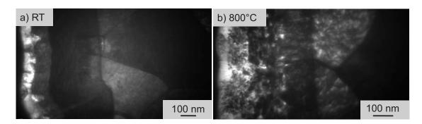
**Figure 6.9:** TEM images of the cross-sections of the stepwise graded W/Cu coating on W fiber a) as-deposited and b) annealed at 800°C.
