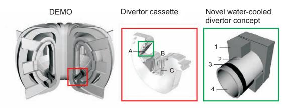
Figure 1.1: Cut-away view of the fusion power core of future fusion reactors with the divertor cassette comprising of A) outer vertical target, B) dome and C) inner vertical target. In the second blow-up the novel optimized water-cooled monoblock divertor concept is presented including 1) W plasma-facing material, 2) brazing foil 3) W<sub>f</sub>/Cu MMC and 4) CuCr1Zr cooling tube (revised from [8])
