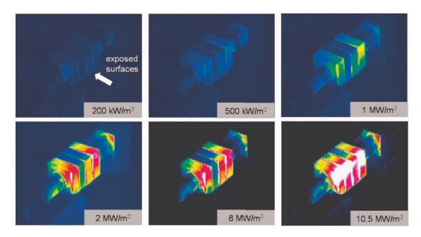
**Figure 8.5:** Infrared camera images during heat flux pulses at different power densities, identifying the hot spots on the monoblock and indicating the highest temperature load at the edges of the W tiles.
