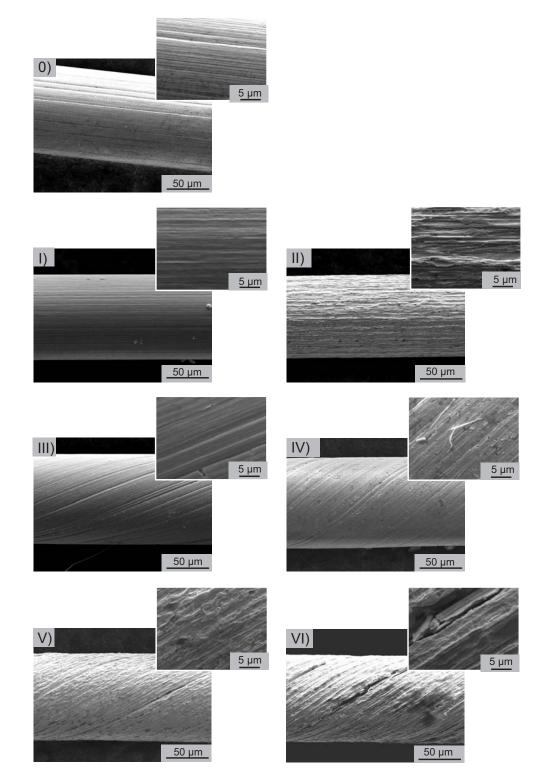
Figure 6.13: SEM images of an initial fiber and of six microstructuring concepts: I) ion sputtering, II) chemical etching, III) fiber twisting to 20°±4°, IV) fiber twisting to 30°±4°, V) fiber twisting to 20°±4° plus chemical etching and VI) fiber twisting to 30°±4° plus chemical etching.
