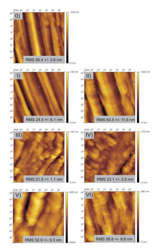
Figure 6.14: 4 μm x 4 μm AFM images of the initial tungsten fiber and of the six microstructuring concepts: I) ion sputtering, II) chemical etching, III) fiber twisting to 20°± 4°, IV) fiber twisting to 30°± 4° V) fiber twisting to 20°± 4° plus chemical etching and VI) fiber twisting to 30°± 4° plus chemical etching. The lines indicate the position of the extracted cross-sectional profiles of Figure 6.15.
