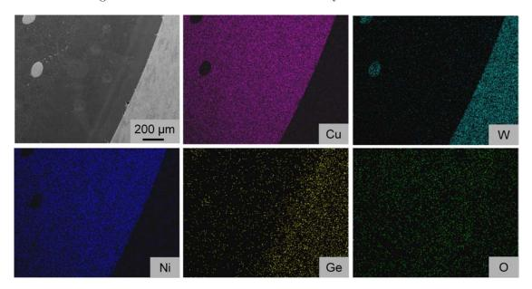
GEMCO brazing foil into Cu while Ge diffused mainly into W.
