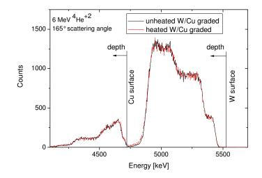
**Figure 6.7:** RBS spectra of unheated and heated (650°C) stepwise graded transition from 100% W to 100% Cu
