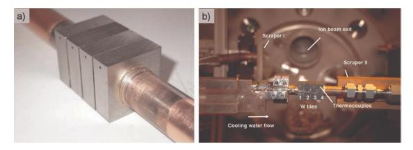
Figure 8.1: a) Finalized optimized monoblock mock-up after the syntheses processes b) Experimental set-up of the monoblock mock-up within the GLADIS vacuum chamber
