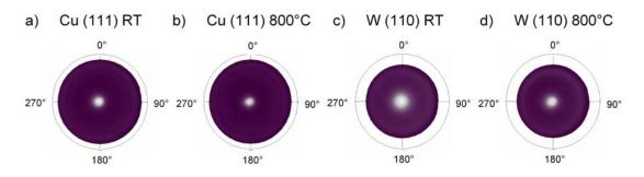
Figure 6.11: Pole figures of the Cu (111) peak of the stepwise graded W/Cu coating on planar W substrates a) as-deposited and b) annealed at 800°C. Pole figures of the W (110) peak of the stepwise graded W/Cu coating on planar W substrates c) as-deposited and d) annealed at 800°C.
