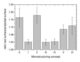
**Figure 6.17:** Comparison of the surface enlargement of the six different microstructuring concepts against the initial fibers. Derived from the average of the  $4 \ \mu m \ x \ 4 \ \mu m$  and  $2 \ \mu m \ x \ 2 \ \mu m \ scanned \ areas.$
