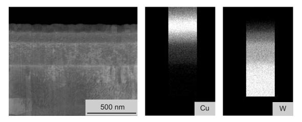
**Figure 6.3:** Resolved Cu and W signal of stepwise graded W/Cu coating (interface concept concept C) measured by EDX
