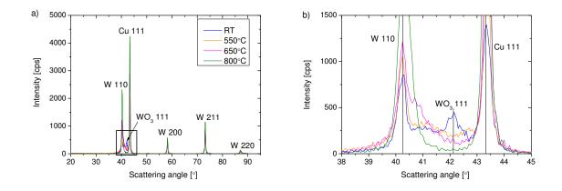
**Figure 6.10:** a) X-ray diffraction pattern of graded W/Cu initial and after heat treatments at 550 °C, 650 °C and 800 °C with its magnification b) showing the disappearance of the WO<sub>3</sub> (111) peak after heating at 550 °C.
