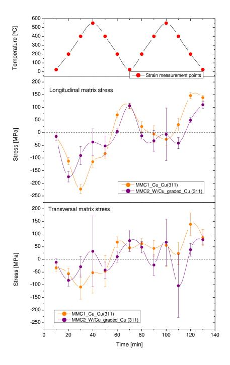
Figure 6.22: Residual stresses of matrix of MMC 1 (composite with initial W fibers with Cu<sub>PVD</sub> interlayer) and of MMC 2 (composite with initial W fibers with continuously graded W/Cu<sub>PVD</sub> without 800°C heat treatment) in longitudinal and transverse direction measured by neutron diffraction
