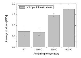
Figure 6.12: Biaxial residual stress state of rotational symmetry of W within the stepwise graded W/Cu coating on SiO<sub>2</sub> after thermal treatments. The stress state was determined based on the W (321) peak
