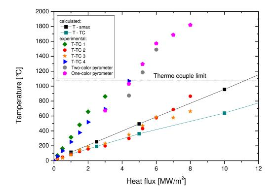
Figure 8.4: Experimental measured temperatures of infrared camera, pyrometer and installed thermo couples within the W tiles #1 - #4 of the  $W_f/Cu$  monoblock mock-up in dependence of different heat fluxes compared with the calculated surface and thermo couple temperature data by FEA
