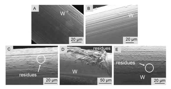
**Figure 6.6:** Failure analysis by SEM images of pulled fibers of single matrix-coated samples with interface concept A, interface concept B, interface concept C, interface concept D and interface concept E
