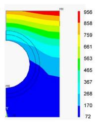
Figure 8.3: Temperature distribution plot of the half cross-section of the monoblock mock-up at a heat flux of 10  $MW/m^2$ . The figure shows the graphical representation of the temperature values of each element within the structure.
