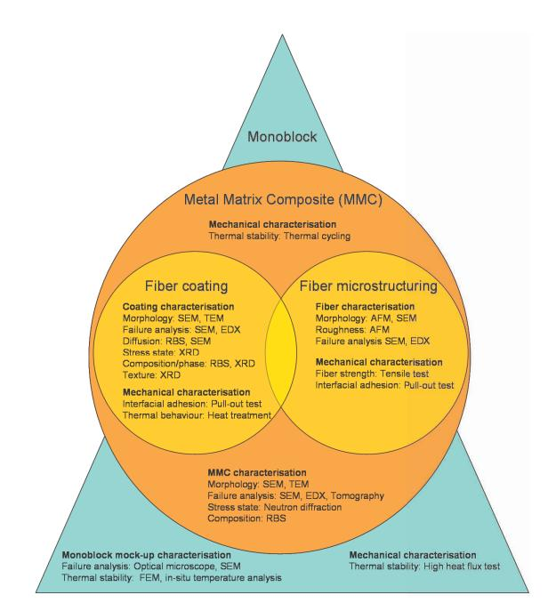
Figure 1.2: The basis of the work is the interface optimization comprising the fiber microstructuring and the fiber coating. Each concept is well characterized and mechanically investigated. The best concepts were unified and applied in the MMC and then implemented into the synthesis of the monoblock mock-up.
