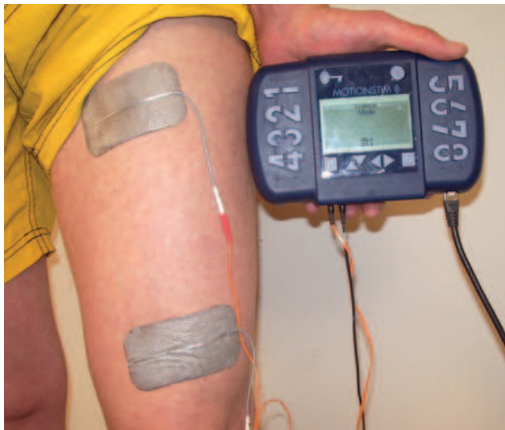
Figure C.1: The stimulator MOTIONSTIM8 from Krauth+Timmermann is used for transcutaneous stimulation of the quadriceps muscle group, which is responsible for knee extension, and hamstring muscles (on the back of the leg), which are responsible for knee flexion.
