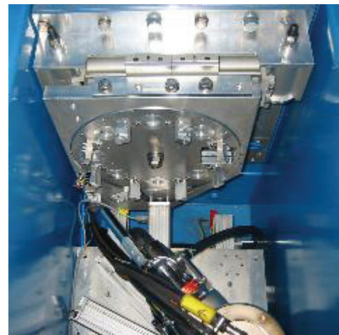
Fig. 2.7: The installed aperture wheel with the 320keV X-ray tube right downstream of it.
