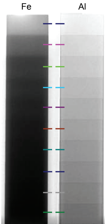
Fig. 3.37: Comparison of the contrast at the edges of an iron and an aluminum step wedge in a phase contrast radiograph. The colored lines represent the positions of the line profiles displayed in Fig. 3.38/39.
