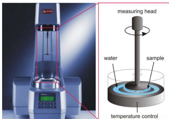
Figure 2.5: Measuring setup of the macrorheometer Physica MCR 301. A measuring head with a plate-plate geometry and 160 mm plate separation is used for all measurements shown in this thesis.
