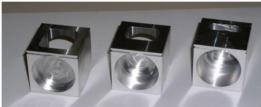
Figure 2.5: Three of the four deuterium target cells with 30, 20, 10 mm thickness, respectively for the neutron beam. The 5 mm target cell is not shown. The cold neutron entrance window can be seen in the front, the hole for the UCN extraction foil in the back.
