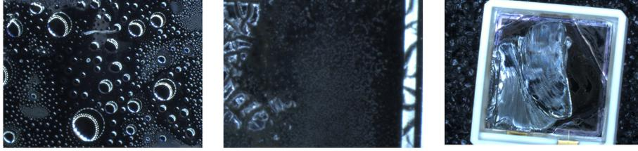
Figure 10.6: LAAPD from Hamamatsu [159] with transparent glue as bought on stock. The glue was removed by bathing in acid. Shown are failures due to strong and to weak acids.
