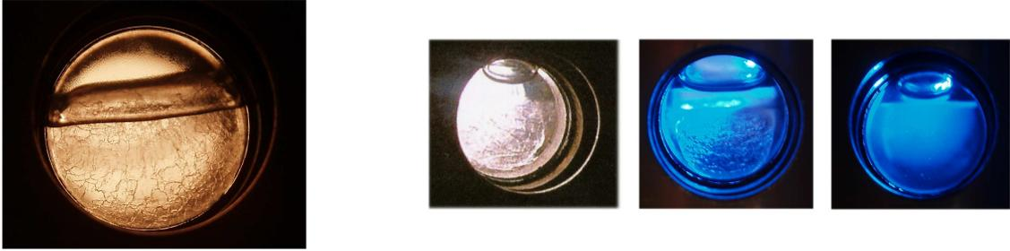
Figure 2.20: Crystal prepared by direct condensation at lowest temperature  $T_{\text{cell}}=8$  K from the gas phase with high over saturation on the left side. Melting of the gas crystal left as a function of time  $\approx 10$  min at  $T_{\text{cell}}=22$  K. The crystal melts in vertical layers and from the top.
