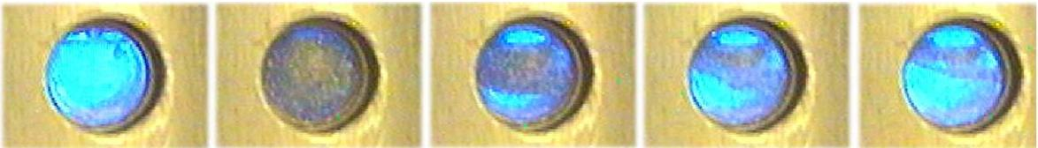
Figure 2.21: Phase transition from liquid (first picture) to solid (second picture) with maximum undercooling: turbo freezing. After moderate turbo freezing, effect of annealing at an intermediate temperature  $T_{\text{cell}}=16K$  shown as function of time (three pictures on the right with a time difference of 1h.)
