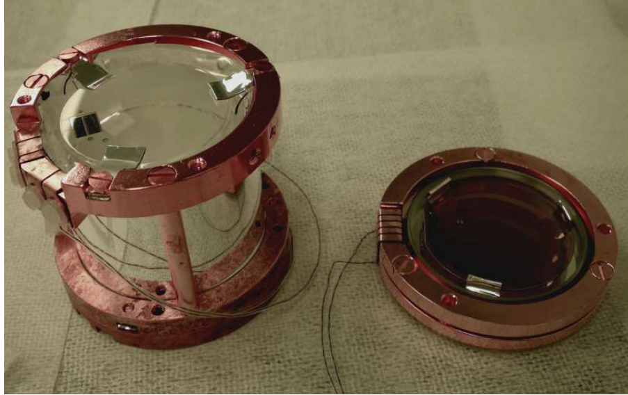
Figure 2.12: Picture of an open detector module for CRESST phase II (Run29 and Run30).
