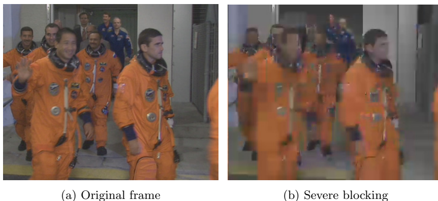
Figure 4.3: Severe blocking as a result of insufficient reproduction of details and block wise motion compensation
