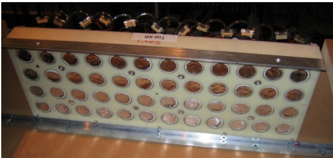
Figure 3.34: Absorber elements covered by aluminum tape on test rig
